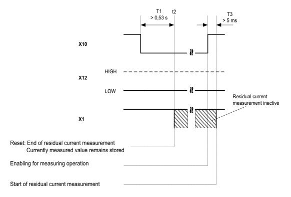
A RESET of the residual current monitoring module RCMB100 can be carried out at any time via the control input X10. In this case, the residual current measurement process has to be interrupted.
