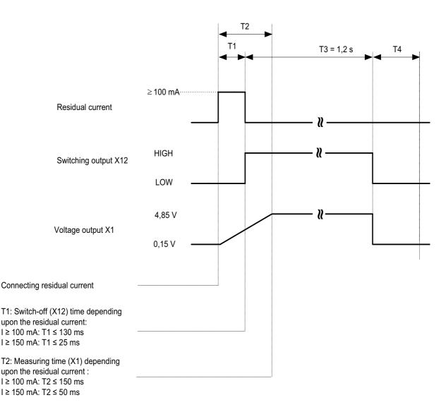
If the residual current exceeds the measuring range (residual current  $\geq$  100mA), the residual current monitoring module RCMB100 will switch the Open-Collector output to HIGH once the measuring time T1 has elapsed.
