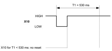
When the condition is met that a LOW level is applied across the control input X10 for at least T1 = 530 ms, disturbing pulses will not cause a RESET of the residual current monitoring module.
