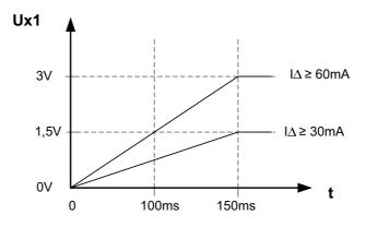
Switching times at the switching output X12:
